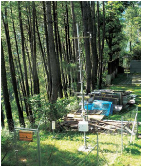
Fig 1.6: Automated Weather Station for recording rainfall, temperature and pressure at DGBR office, Tekhla
