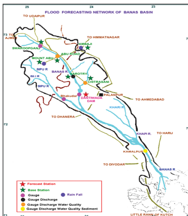
Figure 4: Flood forecasting network of Banas river (Source: CWC 2018) CWC: central water Commission (2018). Hydrological data (unclassified) book
